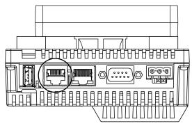
Do not confuse the RJ45 serial port with the RJ45 Ethernet connector.
