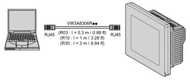
To connect the controller to the PC, do the following:
