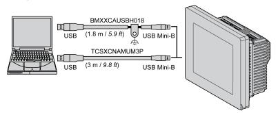
To connect the USB cable to your controller, do the following:
