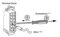
(1) Wire should be 0.20...0.81 mm<sup>2</sup> (AWG 24...18), with the end twisted. Applicable wire sizes are UI 1015 and UI 1007.
