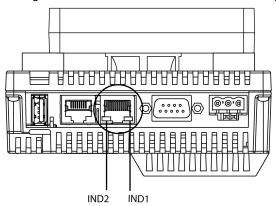
Do not confuse the RJ45 Ethernet connector with the RJ45 serial port.
