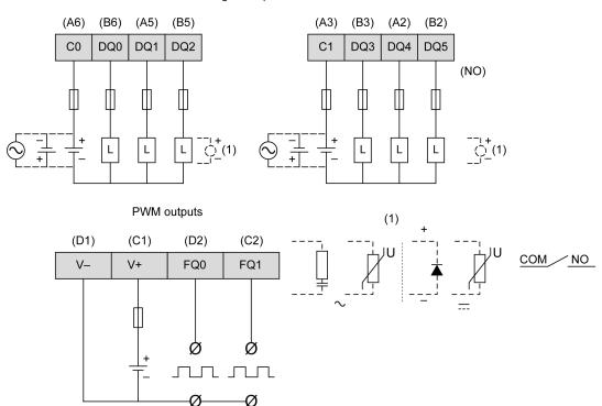
To improve the life time of the contacts, and to protect from potential damage by reverse EMF when using inductive load, connect:
