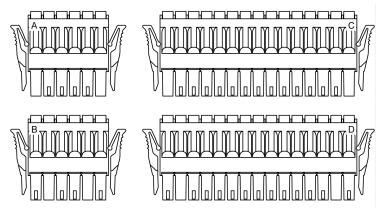
**NOTE:** Terminal blocks A, B, C, and D can only use the respective connectors A, B, C, and D.
