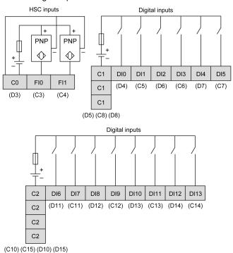
NOTE: The digital inputs are sink type (positive logical).
