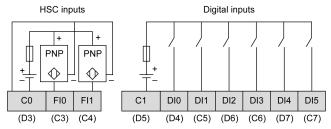
**NOTE:** The digital inputs are sink type (positive logical).
