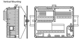
**NOTE:** Keep adequate spacing for proper ventilation to maintain an ambient temperature between 0...50 °C (32...122 °F) for vertical installation and 0...40 °C (32...104 °F) for horizontal installation (face down position).
